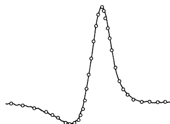
FIG. 14. Line shape of the derivative of the CESR power absorption in film 3 at 4.2 °K. Increasing H_0 is from right to left. The circles are theoretical points including corrections for the anomalous skin effect.
